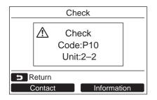
When an error has occurred in the air conditioner, the check code and the unit number of the indoor unit appear on the display of the remote controller.
